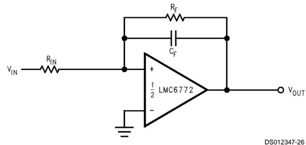
**FIGURE 3. Canceling the Effect of Input Capacitance**
