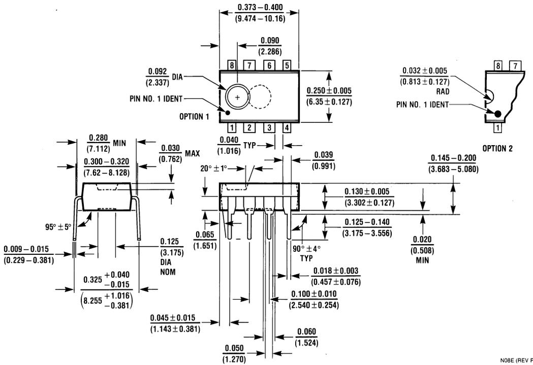
**8-Pin Molded Dual-In-Line Package**
