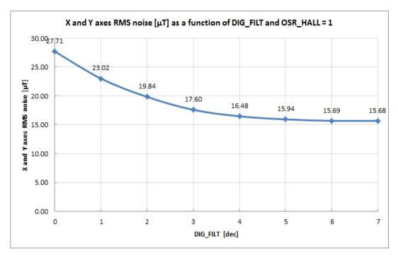
Figure 20: version 011 - XY axis RMS noise (typ)
