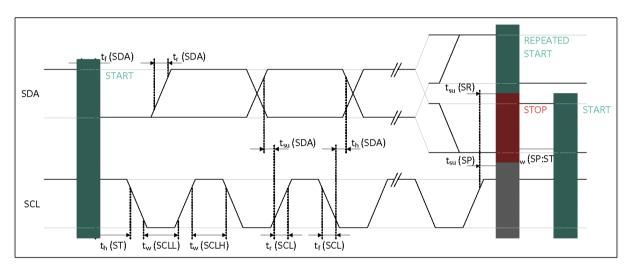
Figure 2: I<sup>2</sup>C Timing Diagram
