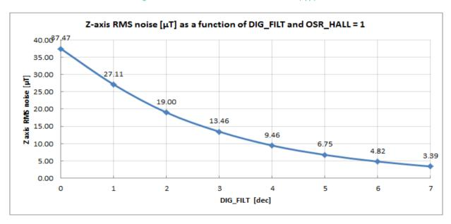
Figure 19: version 011 - Z axis RMS noise (typ)
