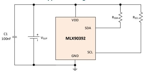
Figure 22: Recommended application diagram
