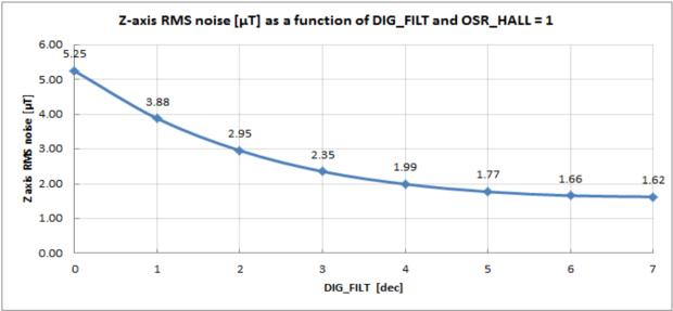
Figure 17: version 010 - Z axis RMS noise (typ)
