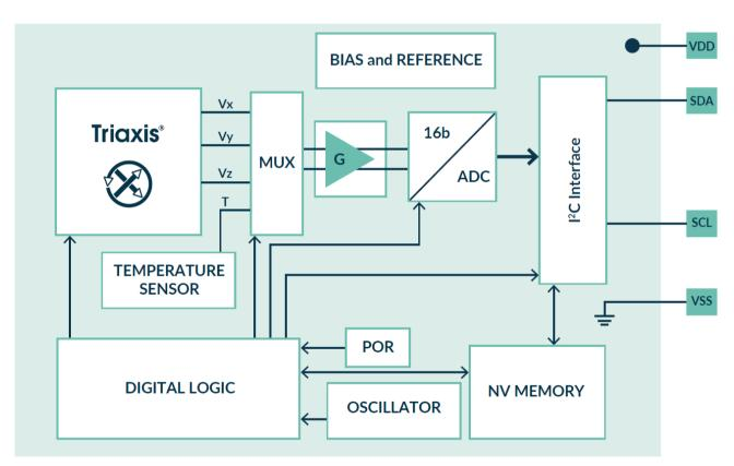
Figure 1: IC block diagram
