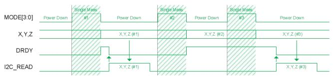
Figure 4: Single measurement mode when data is read out of measurement period
