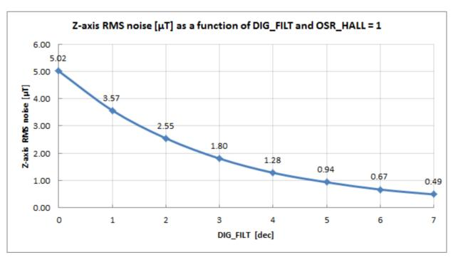
Figure 15: version 010 - Z axis RMS Noise (typ)
