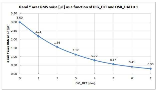
Figure 14: version 010 - XY axis RMS noise (typ)
