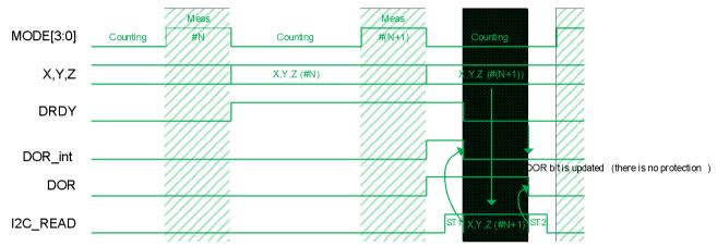
Figure 9: Data Skip: When data is not read
