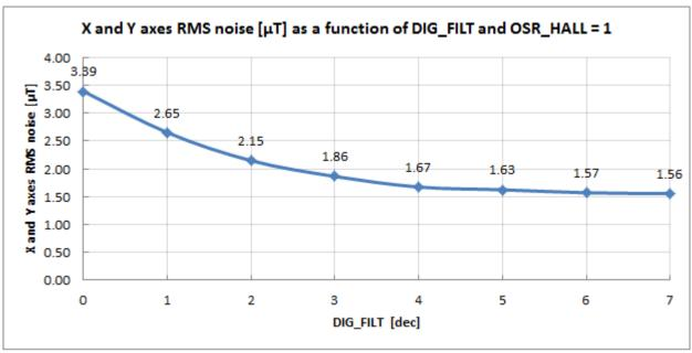
Figure 16: version 010 - XY axes RMS noise(typ)
