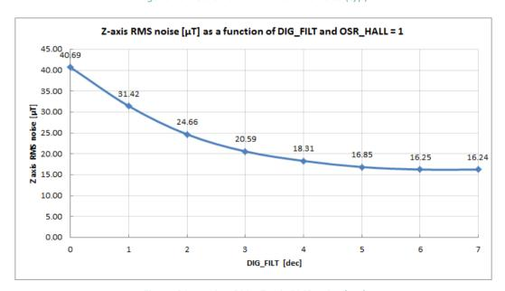
Figure 21: version 011 - Z axis RMS noise (typ)
