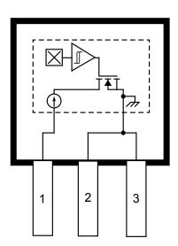
LH Package, 3-Pin SOT23W Pinout
