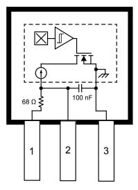
UC Package, 3-Pin SIP Pinout
