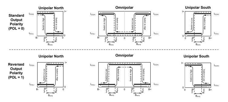
Figure 1: Hall Switch Magnetic and Output Current Polarity Options B- indicates increasing north polarity magnetic field strength, and B+ indicates increasing south polarity magnetic field strength.
