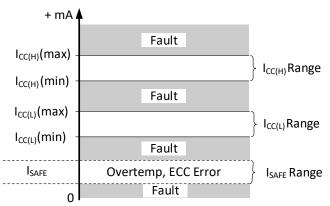
Figure 5: Interpreting I<sub>CC</sub> for System-Level Diagnostics
