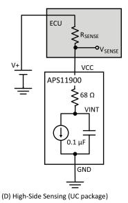
**Figure 6: Typical Application Circuits**
